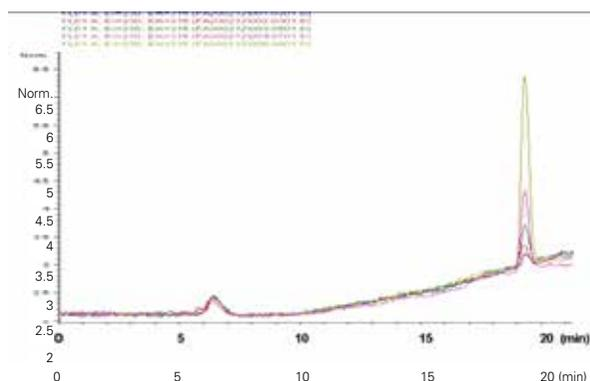
**Figure 1.** High-performance liquid chromatography (HPLC) chromatogram of bisphenol A (BPA) standards. Calculations were made according to the peak heights. Retention times were between 18.3-19.2 minutes
